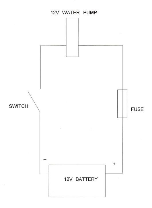
E-Z BUILT HOT DOG CART Wiring Diagram www.HotDogProfits.com
